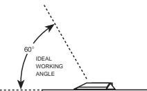
The microphone should be placed on a flat, unobstructed mounting surface, with the front of the microphone facing the sound source. The sound source should not be below, or higher than 60° above, the plane of the mounting surface.
